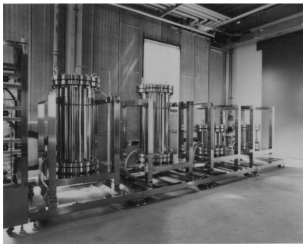
FIG. 1. Photograph of columns for industrial preparative high-performance liquid chromatography.
